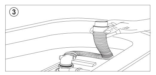
• If you have a waste that comes up through the floor, you can connect to it with a flexible drain pipe which enables you to tilt the bath up and move the bath into the required position. To avoid water retention in the trap the flexible pipe should have a continuous downward flow.
